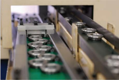
After an operator loads the parts onto the LZ-01R's conveyor, the process is fully automated.
