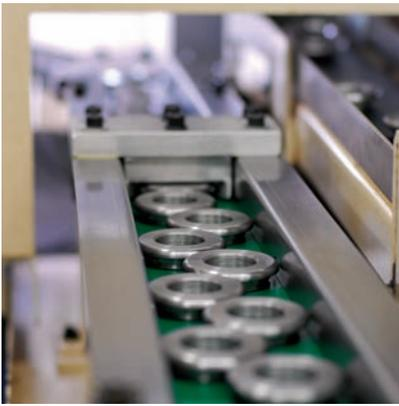
When companies need large volumes of accurately machined parts to meet their production requirements, they turn to one of the most reliable CNC turning centers available: the Miyano LZ-01R automated chucker. The very best in machining technology, the LZ-01R combines precision and speed to turn parts up to 3 1/2" in diameter and up to 1 1/2 lbs.
